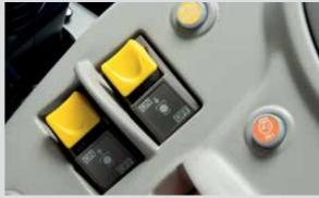
Electro-hydraulic switches to engage PTO.
