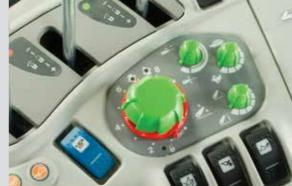
Console with electronic hitch control
