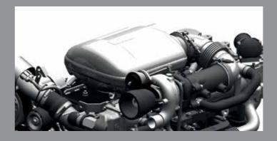
DOC - (Diesel Oxidation Catalyst): The exhaust gas oxydation catalyst (DOC) helps reduce pollutants via a "catalytic sponge". It converts the unburned hydrocarbons (HC), the nitrogen oxides (NO) and the carbon monoxide (CO) into carbon dioxide, nitrogen and water in the form of water vapour. Unlike diesel particulate filters (DPF), the DOC remains effective throughout the service life of the engine without any need for regular maintenance or active regeneration.
