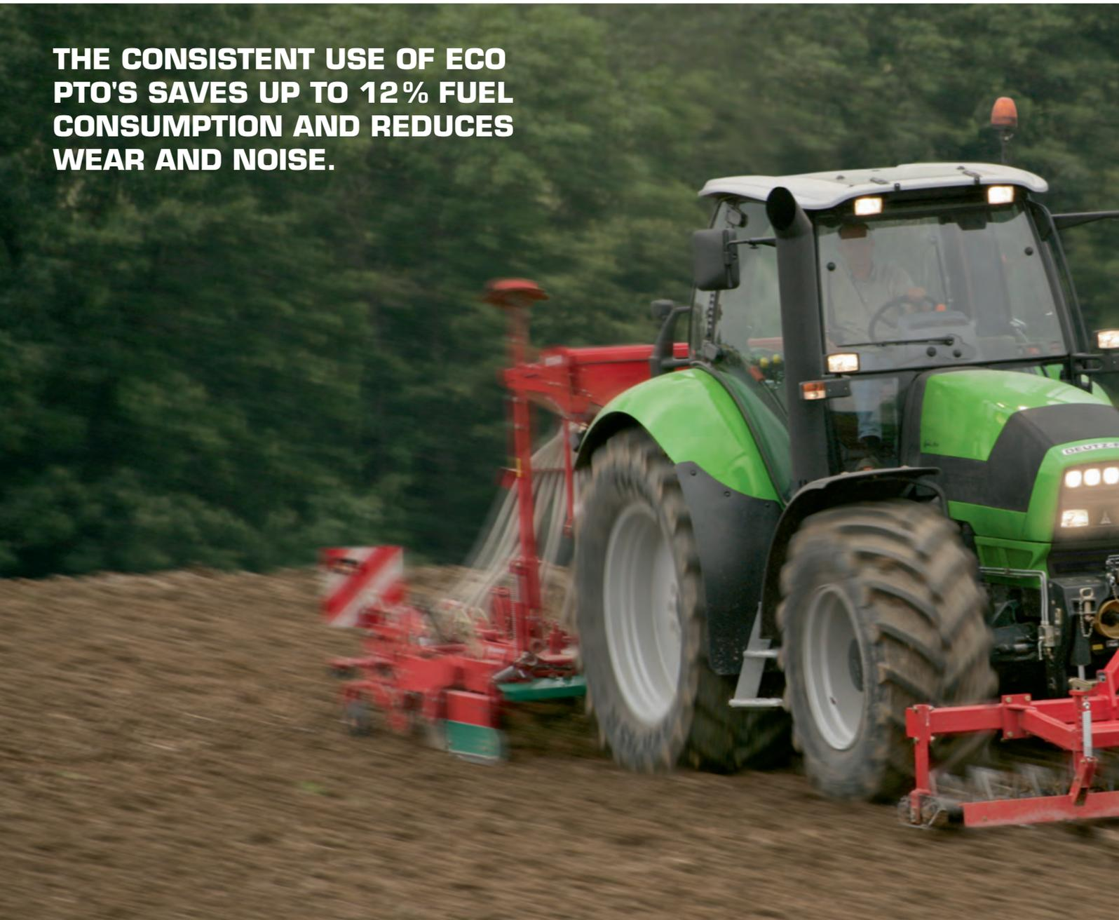
**The Agrotron is one of the few tractors in its class to have a four speed rear PTO as a standard feature: (540/540 E/ 1,000/1,000 E rpm) effectively covering a wide range of applications.**
