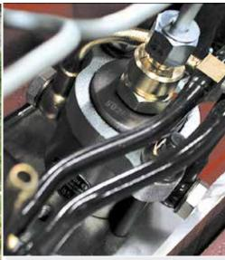
Optimum fuel utilization thanks to the 5-hole injection nozzles.
