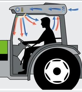
Heating, ventilation and air conditioning (upon request) are located in the cab roof.
