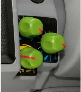
The Electronic Hitch Regulation can be adjusted quickly and easily with rotary regulators.
