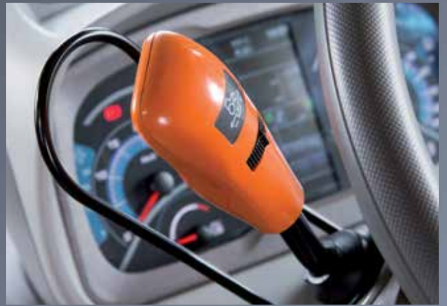
Electro-hydraulic Powershuttle SenseClutch for precise and safe changes of direction while driving and with load without interruption of torque.
