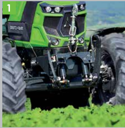
Hydraulic packages with 22 equipment options, e.g. a front linkage with ComfortPack.
